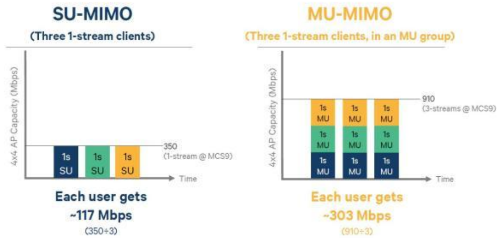
Figure 4-6 Throughput difference between SU-MIMO and MU-MIMO
