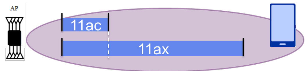
Figure 4-13 Range increase brought by long OFDM symbol and narrowband transmission
