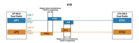
The AP MLD and STA MLD are dual-radio MLDs, and can transmit UL and DL frames asynchronously on Link 1 and Link 2 at the same time
