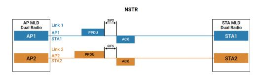
The AP MLD and STA MLD can transmit and receive simultaneously on Link 1 and Link 2, but cannot transmit on one link while receiving on another
